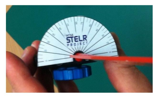
**Tip:** Check that all blades have been angled in the same direction before attaching to the turbine.
