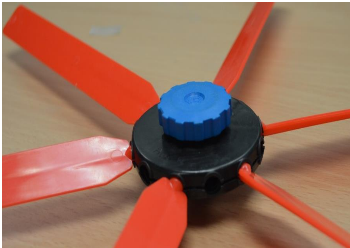
Figure 2: These blades have been set into the hub at the same angle ( 45^{\circ} )
