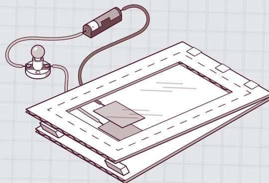
Here's one of many ideas for making a dance pad. When you apply a force, plastic wrap stretches. It returns to its original shape once you remove the force. Its springiness and flexibility can be useful in making a switch.
