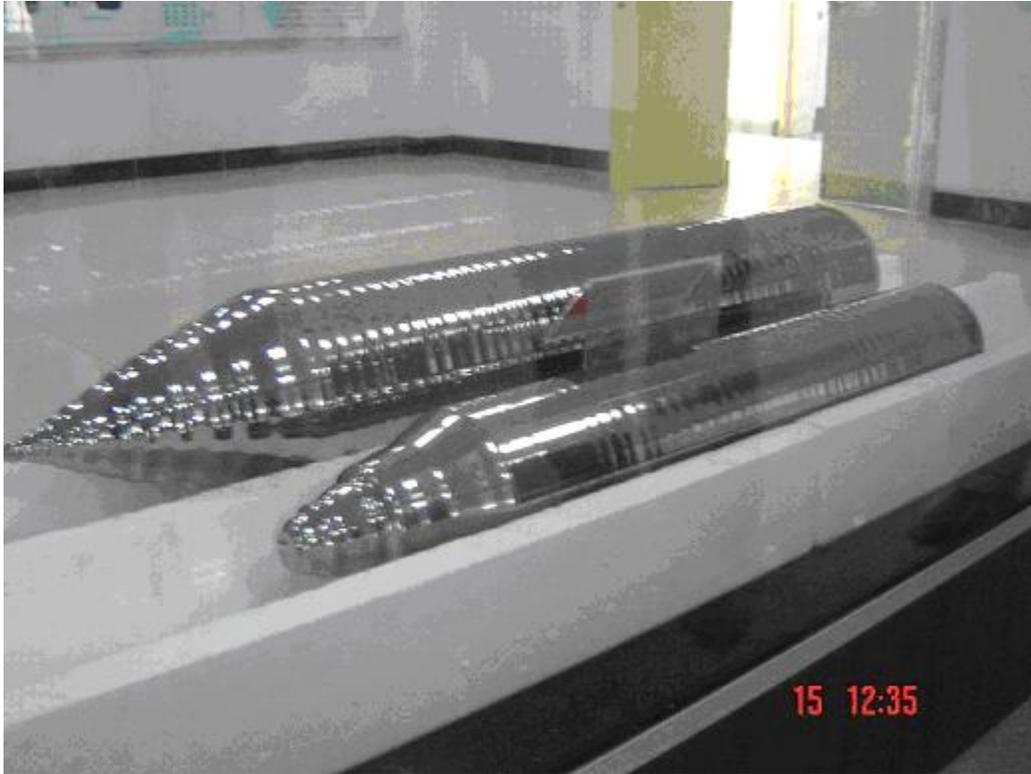
Figure 9: Silicon ingots prior to sawing into wafers. Each ingot is a single crystal
