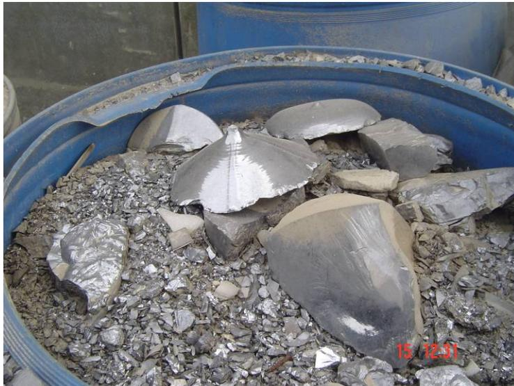
**Figure 26:** A drum of scrap silicon chips awaiting re-melting and growth into ingots for later sawing into wafers for solar cell manufacture
