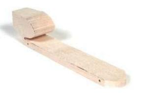
2. Smooth the corners of your car body. Use a bench-mounted sander, sharp knife, wood rasp, files, or rough sandpaper (80 grit) to smooth the car to its basic rounded shape.
