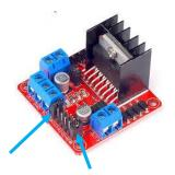
You will need to remove the jumpers from the L298N motor controller.
