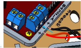
6. Insert wires into blue terminals.
