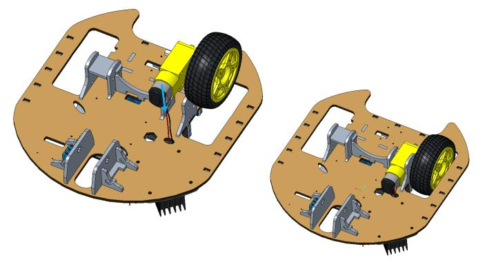
13. Feed the long wires through the oval hole. Push the yellow gearbox into place.The long wires go through the long oval.Don't forget to to lock it in with the bread.
