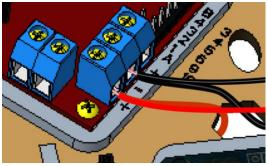
P o w e 7. Plug the **black** wire into the **GND** socket on the Arduino. Plug the red wire into the **VIN** socket on the Arduino.
