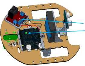
Now is a good time to test the power circuit. Put in 4 AA batteries and switch the robot on. A red light should light up on the motor controller and a green or red light on the arduino.
