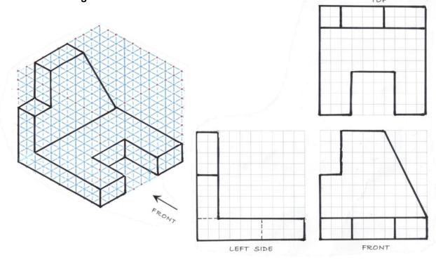
Q2 Taking the dimensions from the isometric view, sketch the top, front and side orthogonal views.
