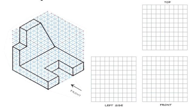
Q2 Taking the dimensions from the isometric view, sketch the top, front and side orthogonal views.
