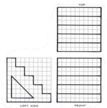
Q2 Taking the dimensions from the isometric view, sketch the top, front and side orthogonal views.
