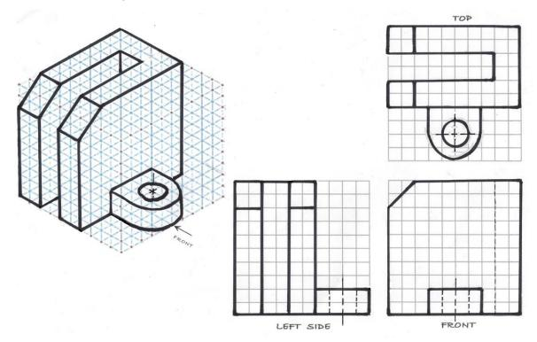
Q2 Taking the dimensions from the isometric view, sketch the top, front and side orthogonal views.
